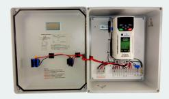
The ImPulse Controller varies the milk pump speed in order to pump the milk through a plate cooler as slowly as possible while still keeping up with milk inflow in the receiver. Usually the pumping rate is significantly less than the maximum, so the cooling efficiency of the plate cooler is increased, resulting in reduced electrical needs for refrigeration.
