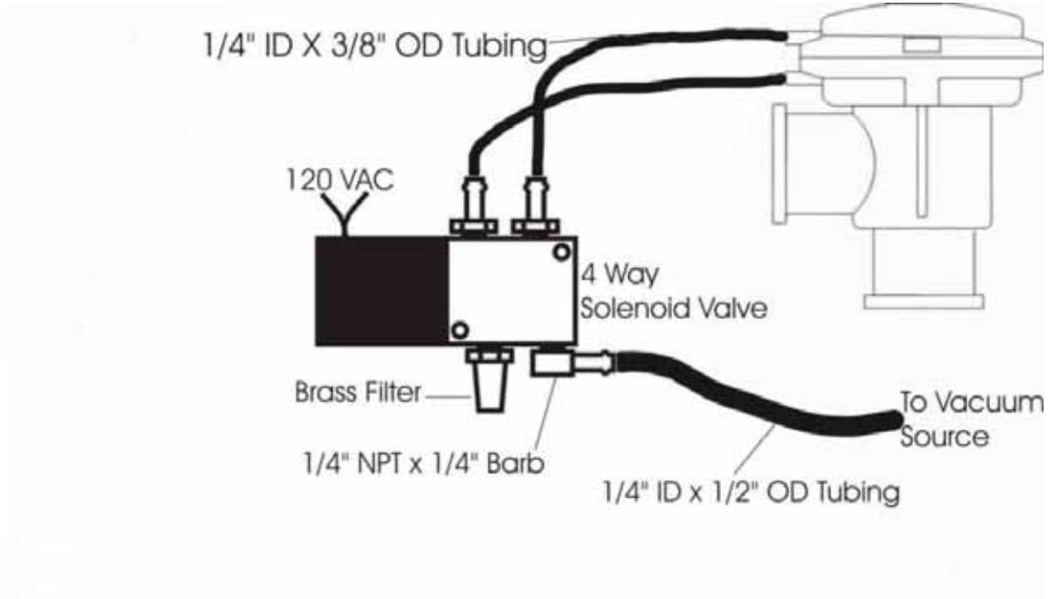
**Figure 4** Wiring Diagram
