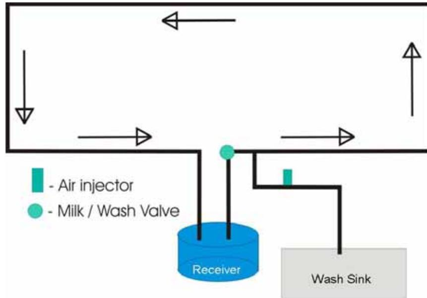
**Figure 6** - Around the Barn Pipeline—2 Equal Loops
